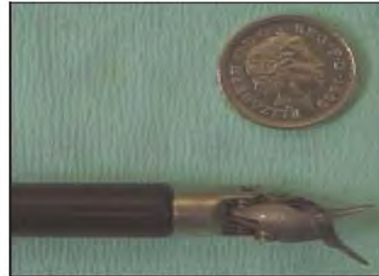
Fig 3 Effector tips of the da Vinci surgical system incorporate miniature wrists that allow them to mimic any movement made by the surgeon at the control console
