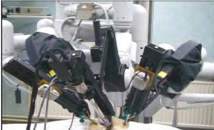
Fig 2 Effector arms of da Vinci surgical system. The attached instruments are controlled by the surgeon, who sits at an adjacent console
